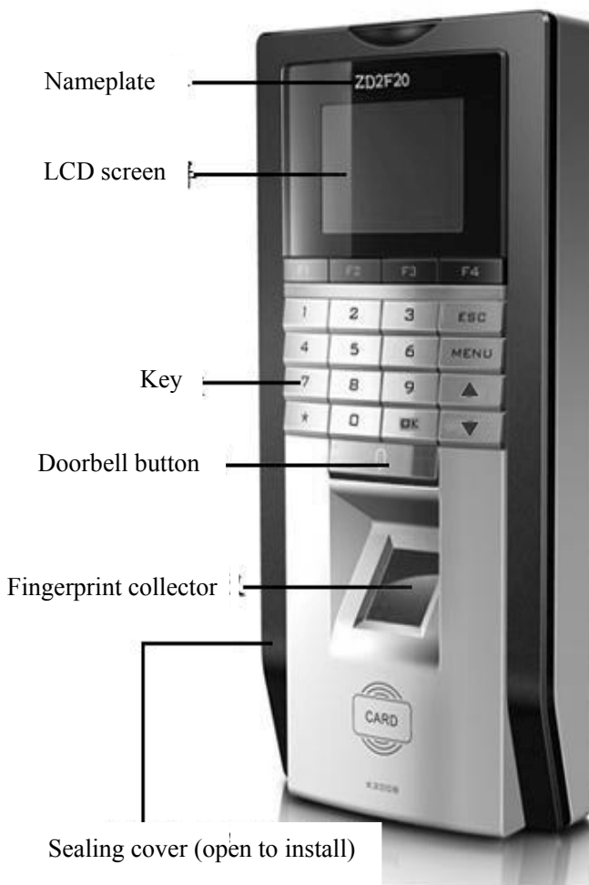
Appearance of the Fingerprint Access Control/Attendance Time Clock (Front)
